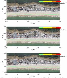
Fig.5. Predicted Wave-RunUp heights according to: (A) Holman (1984) formula; (B) a site-specific formula using video images by Voudouskas (); (C) the Xbeach modelling
