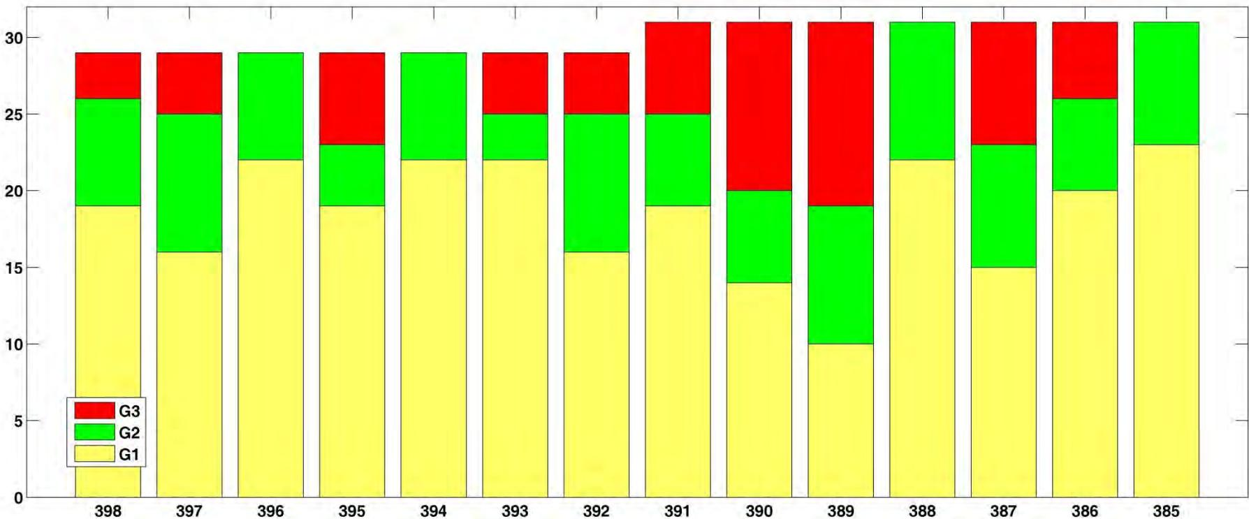
The threshold values of dune erosion for the groups of the storms identified by the Ward's method were obtained using a classification tree.
